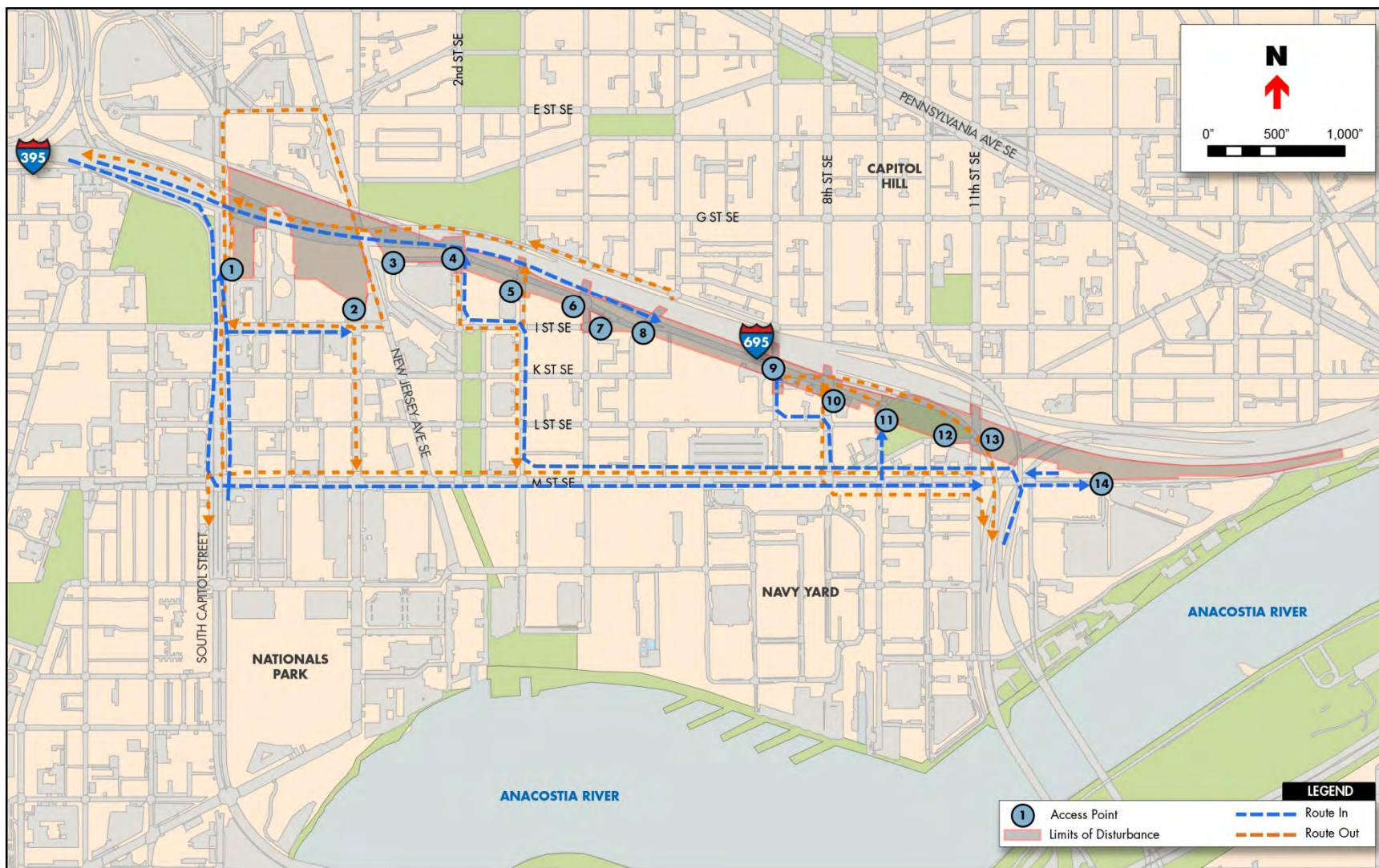
Figure 3-6 Construction Haul Routes and Access Points
